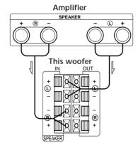
2 Connect the front speakers to the woofer. Connect the speakers to the speaker terminals of the woofer.
